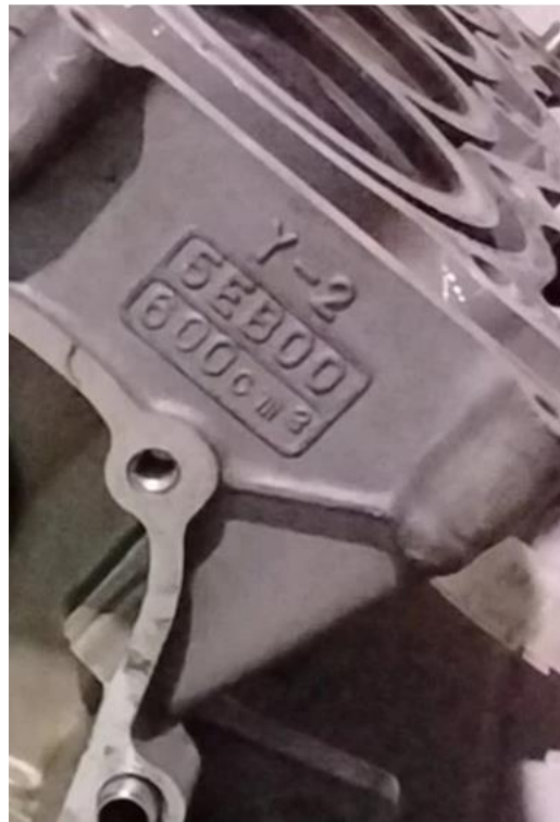
Incorrect 5SL crankcase (not to be used)
