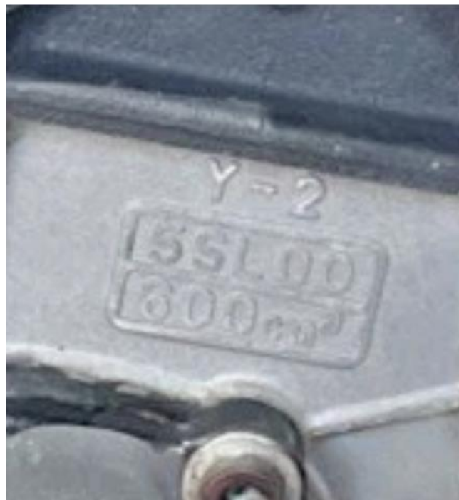
Incorrect 5SL crankcase (not to be used)
